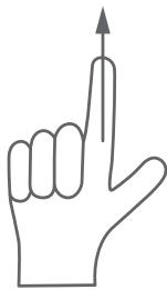
Beginning of rope reeling from the left side of the drum for the right-lay rope
